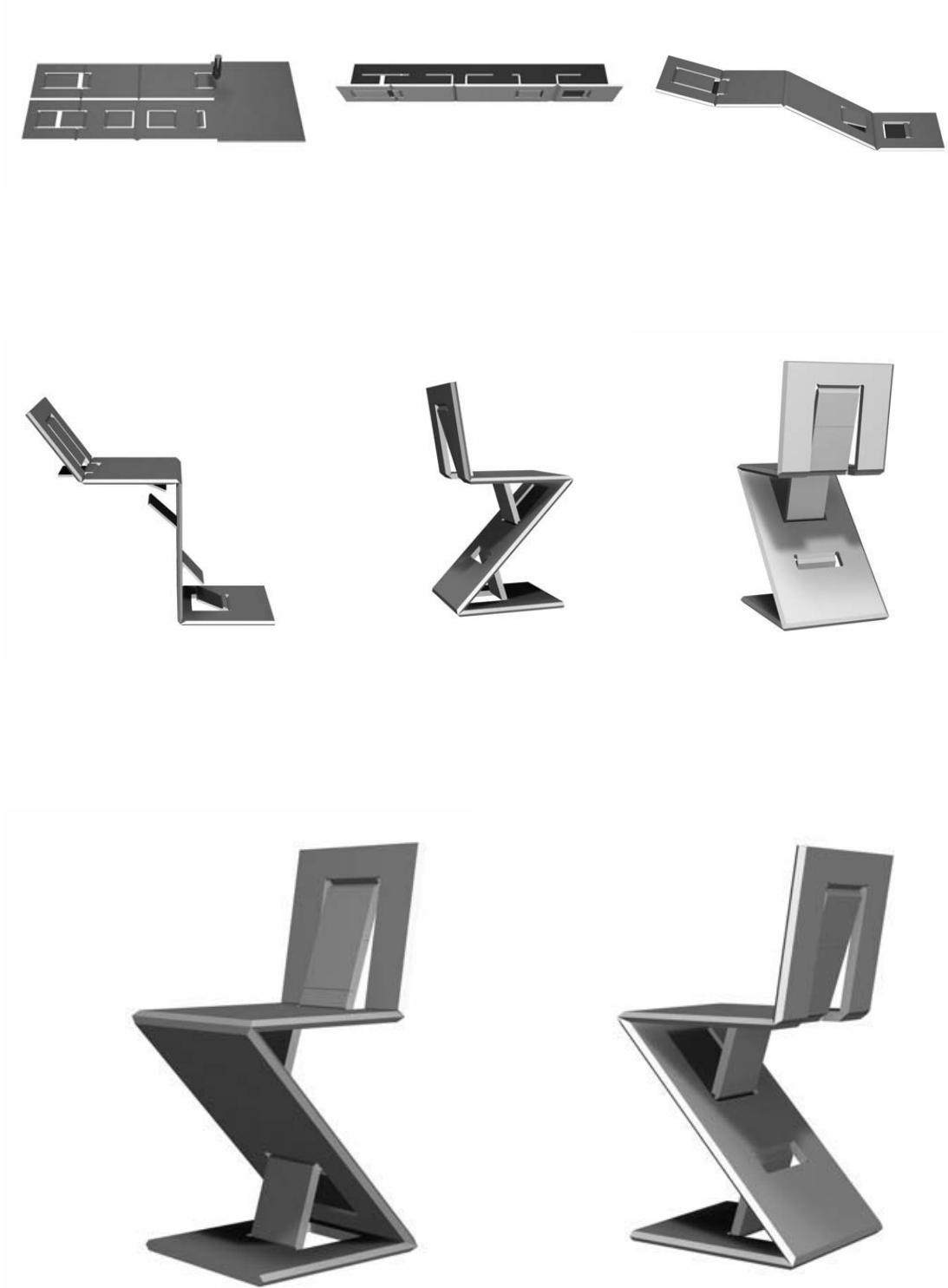
Fig.3: Milling and folding of a chair (Cig-Cag_Chair, Design: J. Gros)
